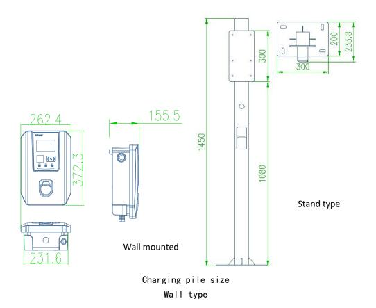
1. Please confirm the installation position and mark it. The center of the charging pile should be at least 1.3m above the ground, as shown in Figure .
